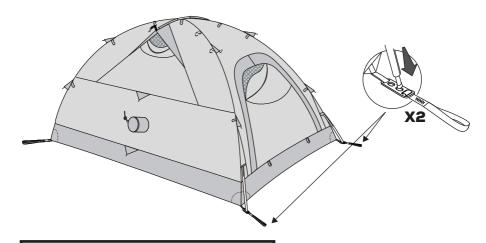
Rise up one pole per time and insert the tip in the outer plate hole.
